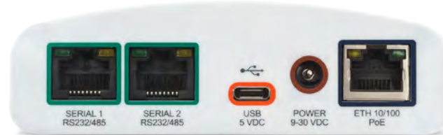
Figure 3-7 Back Panel for non-medical SGX 5150
