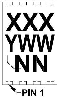
8-Lead MSOP (3x3 mm)
