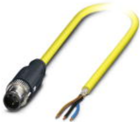
Sensor/Actuator cable, 3-position, PVC, Variable cable type, Yellow RAL 1021, shielded, Plug straight M12-SPEEDCON, A-coded, on Free cable end, Cable length: 5 m
