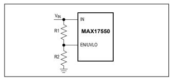
Figure 2. Adjustable EN/UVLO Network
