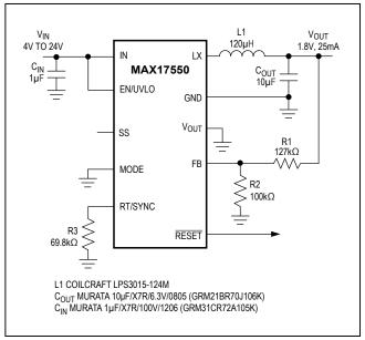
Figure 10. Small-Footprint 1.8V, 25mA Regulator
