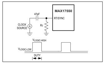
Figure 1. Synchronization to an External Clock
