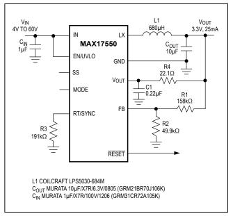
Figure 7. High-Efficiency 3.3V, 25mA Regulator
