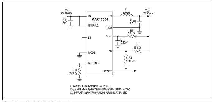
Figure 8. Small-Footprint 5V, 25mA Regulator
