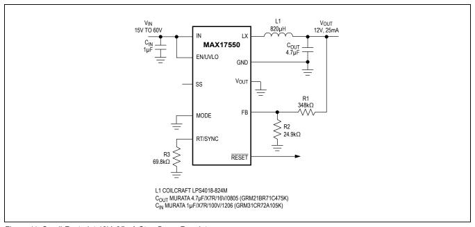
Figure 11. Small-Footprint 12V, 25mA Step-Down Regulator
