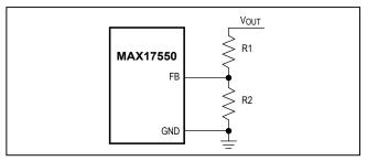
Figure 3. Setting the Output Voltage
