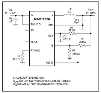
Figure 6. High-Efficiency 5V, 25mA Regulator
