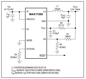
Figure 9. Small-Footprint 3.3V, 25mA Regulator
