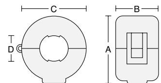
May also be mounted with a flat-head screw through the .120" (3,0mm) diameter hole in the bottom by temporarily removing lower ferrite half.
