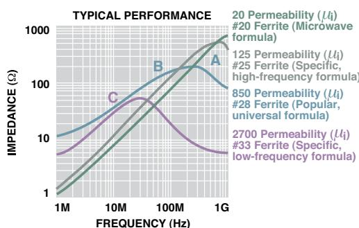
**fig. 1** Typical attenuation profiles
