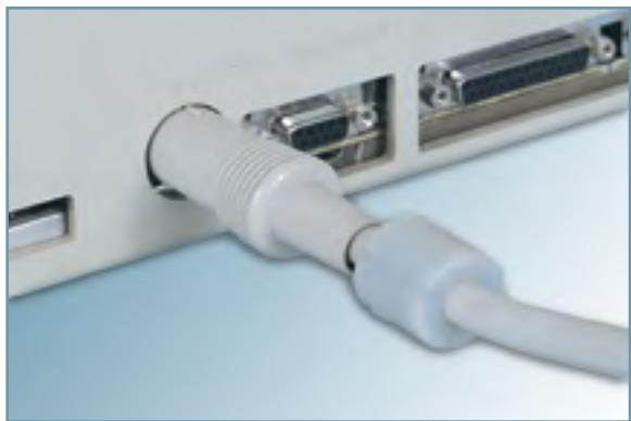
I/O cable with RFI suppressor.
