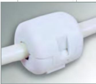
Ferrite assembly in fully enclosed nylon case; functional with wires and cables up to a 2.0" (50,8mm) diameter. Snap closed around wire by clasping shut to position assembly.
