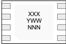
8-Lead DFN (2x3) (MCP4011)
