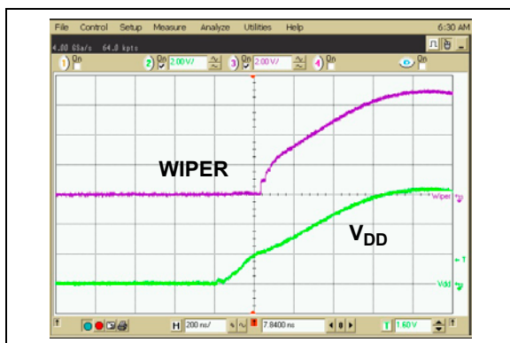
FIGURE 2-15: 2.1 k \Omega – Power-Up Wiper Response Time.
