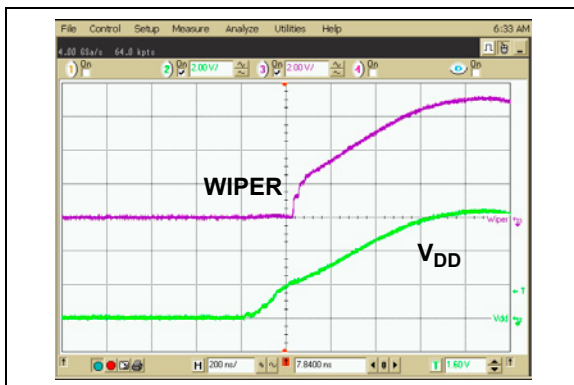
FIGURE 2-52: 50\text{ k}\Omega – Power-Up Wiper Response Time.
