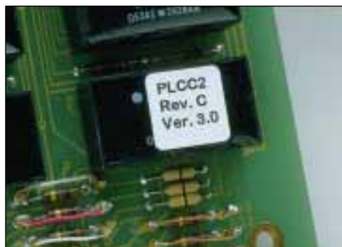
Circuit Board Labeling
