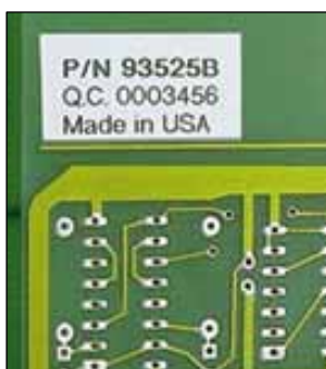
Circuit board labeling
