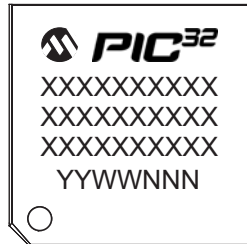
64-Lead TQFP (10x10x1 mm)
