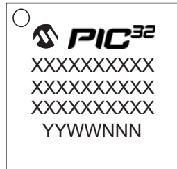
64-Lead TQFP (10x10x1 mm)
