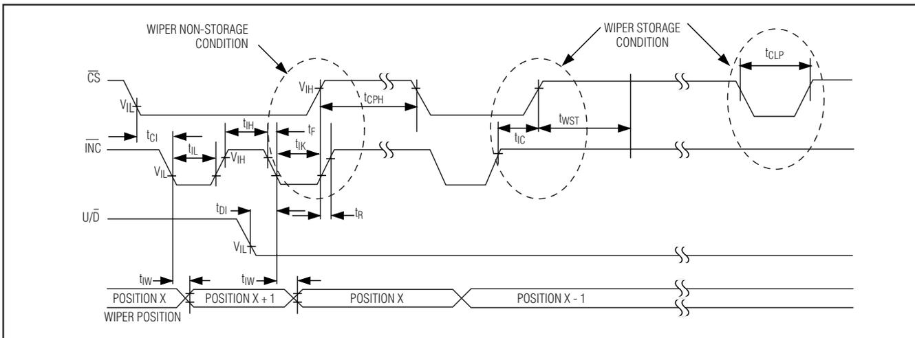
Figure 2. Timing Diagram
