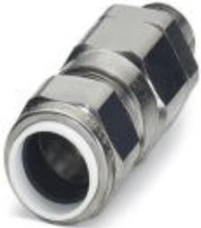
Cable gland, Cable gland material: Nickel-plated brass, Application: Ex, External cable diameter 23.7 mm ... 33.9 mm, Shielding: Yes, Connecting thread: M32, Color: silver
