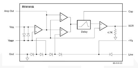
Figure 1. Block Diagram
