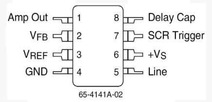
Figure 2. Pin Assignment
