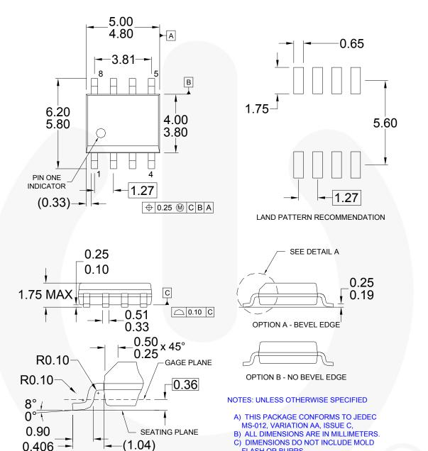
Figure 5. 8-Lead, Plastic Small-Outline Integrated Circuit (SOIC)
