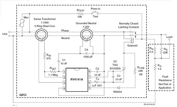
Figure 3. GFI Application Circuit
