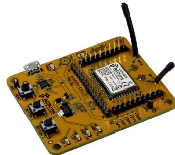
Figure 9 - AMW006-E03 eval board with wire antennas
