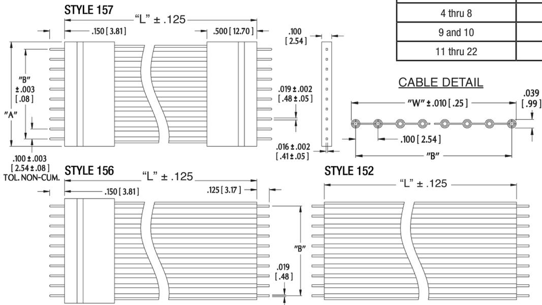
$"A" = (\text{NO. OF CONDUCTORS} \times 0.100 [2.54]) + 0.040 [1.02]$
