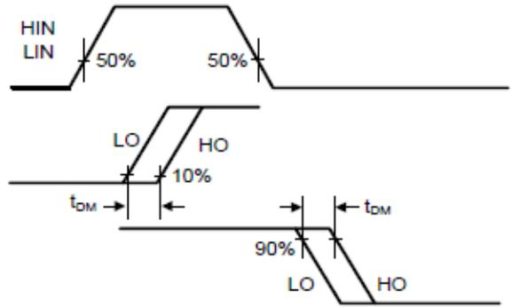
**Figure 2.** Delay Matching Waveform Definitions
