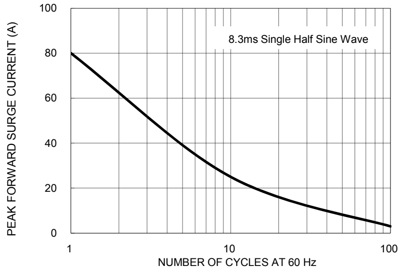
FIG. 3 MAXIMUM NON-REPETITIVE FORWARD PEAK SURGE CURRENT
