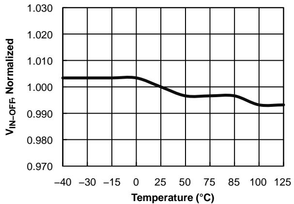
Figure 4. Turn-Off Threshold Voltage ( $V_{IN-OFF}$ ) vs. Temperature
