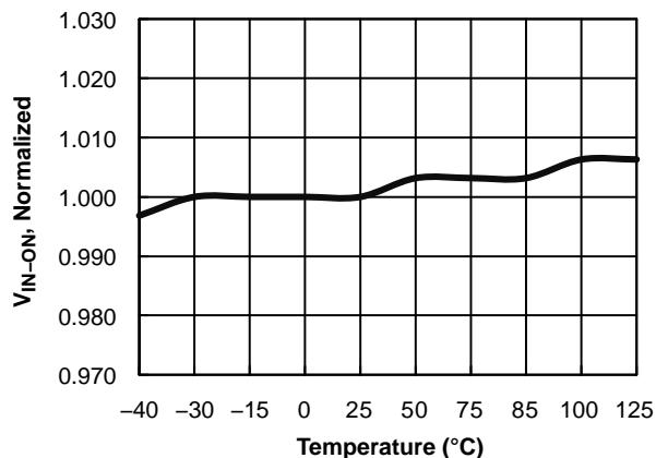
Figure 3. Turn-On Threshold Voltage ( $V_{IN-ON}$ ) vs. Temperature
