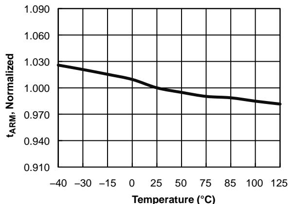
Figure 14. Gate Re-arm Time for Slope Detection (t<sub>ARM</sub>) vs. Temperature
