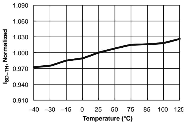
Figure 13. Shut-Down Current Source (I<sub>SD-TH</sub>) vs. Temperature
