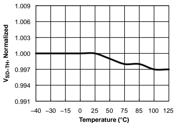
Figure 12. Shut-Down Threshold Voltage (V<sub>SD-TH</sub>) vs. Temperature
