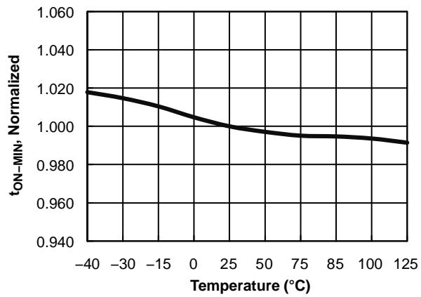
Figure 6. Minimum On Time ( $t_{ON-MIN}$ ) vs. Temperature
