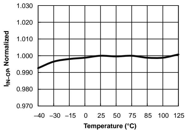
Figure 5. Operating Supply Current ( $I_{IN-OP}$ ) vs. Temperature
