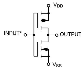
\*Double diode protection on all inputs not shown
