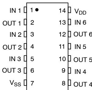
**Figure 1. Pin Assignment**
