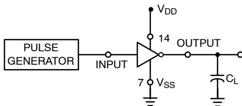
**Figure 4. Switching Time Test Circuit and Waveforms**
