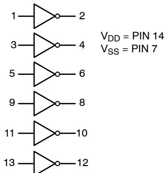
**Figure 3. Logic Diagram**
