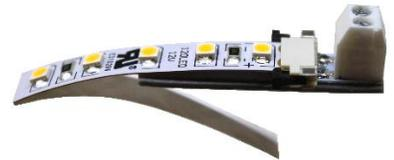
**5** Make sure LED strip is centered and fully inserted before sliding black latch firmly closed and pressing on adhesive
