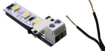
**8** Insert wire (matching polarity) tighten screws and connect to class 2 power source to verify connections, then install LED flex strips as needed
