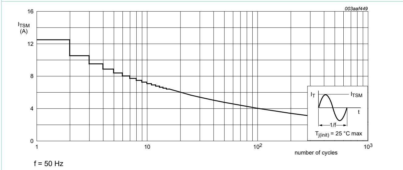
Fig. 4. Non-repetitive peak on-state current as a function of the number of sinusoidal current cycles; maximum values
