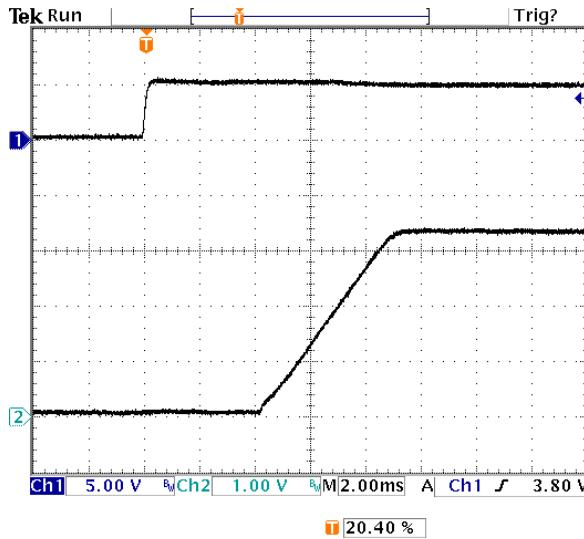
**Fig-3.3V-4:** Turn-on transient for  $V_{out}=3.3V$  with application of  $V_{in}$  at full rated load current (resistive) and  $47\mu Fx2$  external capacitance at  $Vin=5.0V$ .
