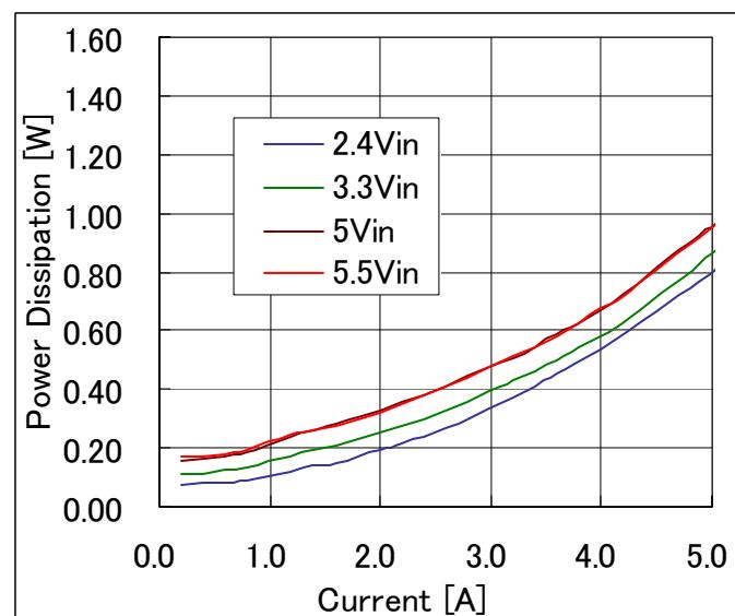
**Fig-0.7525V-3:** Power dissipation vs. load current and input voltage for  $V_{out}=0.7525V$ .
