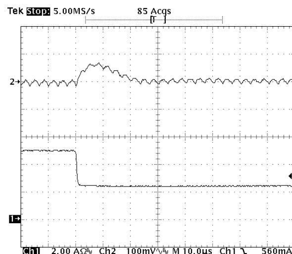
**Fig-1.2V-7:** Output voltage response for  $V_{out}=1.2V$  to positive load current step-change from  $5A$  to  $2.5A$  with slew rate of  $-5A/\mu s$  at  $V_{in}=5.0V$ .  $C_o=47\mu Fx2$  ceramic.
