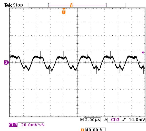
**Fig-1.8V-5:** Output voltage ripple (20mV/div.) for  $V_{out}=1.8V$  at full rated load current into a resistive load with external capacitance  $47\mu Fx2$  ceramic +  $1\mu F$  ceramic at  $V_{in}=5.0V$ .
