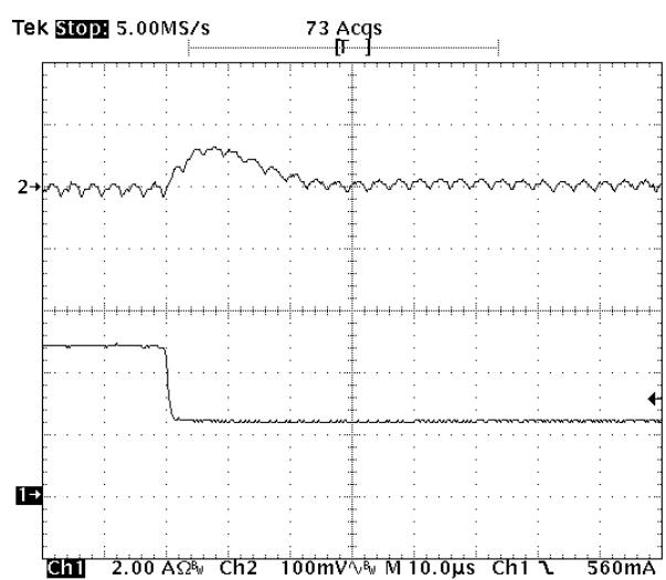
**Fig-1.0V-7:** Output voltage response for  $V_{out}=1.0V$  to positive load current step-change from 5A to 2.5A with slew rate of  $-5A/\mu s$  at  $V_{in}=5.0V$ .  $C_o=47\mu Fx2$  ceramic.
