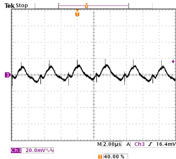
**Fig-2.5V-5:** Output voltage ripple (20mV/div.) for  $V_{out}=2.5V$  at full rated load current into a resistive load with external capacitance  $47\mu Fx2$  ceramic +  $1\mu F$  ceramic at  $V_{in}=5.0V$ .
