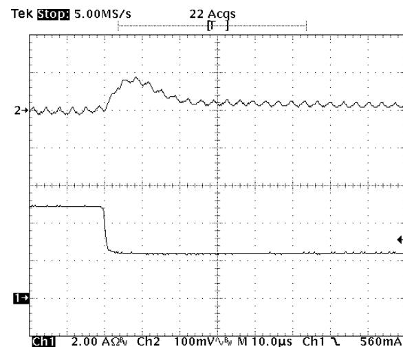
**Fig-3.3V-7:** Output voltage response for  $V_{out}=3.3V$  to negative load current step-change from 5A to 2.5A with slew rate of  $-5A/\mu s$  at  $Vin=5.0V$ .  $Co=47\mu Fx2$  ceramic.
