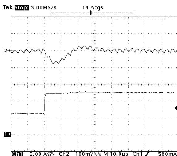
**Fig-1.8V-6:** Output voltage response for  $V_{out}=1.8V$  to positive load current step-change from 2.5A to 5A with slew rate of  $5A/\mu s$  at  $V_{in}=5.0V$ .  $C_o=47\mu Fx2$  ceramic.
