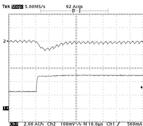
**Fig-1.0V-6:** Output voltage response for  $V_{out}=1.0V$  to positive load current step-change from 2.5A to 5A with slew rate of  $5A/\mu s$  at  $V_{in}=5.0V$ .  $C_o=47\mu Fx2$  ceramic.
