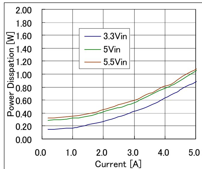
**Fig-2.0V-3:** Power dissipation vs. load current and input voltage for  $V_{out}=2.0V$ .
