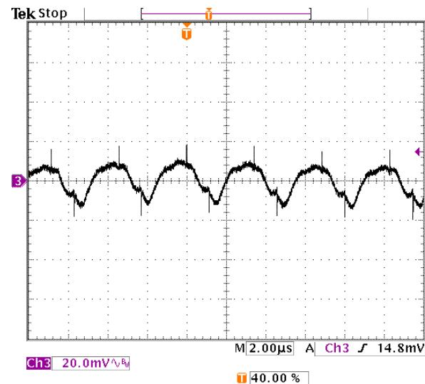
**Fig-1.5V-5:** Output voltage ripple (20mV/div.) for  $V_{out}=1.5V$  at full rated load current into a resistive load with external capacitance  $47\mu Fx2$  ceramic +  $1\mu F$  ceramic at  $V_{in}=5.0V$ .
