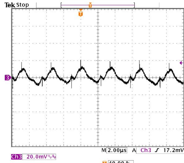
**Fig-3.3V-5:** Output voltage ripple (20mV/div.) for  $V_{out}=3.3V$  at full rated load current into a resistive load with external capacitance  $47\mu Fx2$  ceramic +  $1\mu F$  ceramic at  $Vin=5.0V$ .
