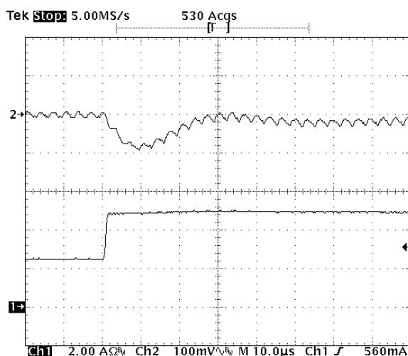
**Fig-2.5V-6:** Output voltage response for  $V_{out}=2.5V$  to positive load current step-change from 2.5A to 5A with slew rate of  $5A/\mu s$  at  $V_{in}=5.0V$ .  $C_o=47\mu Fx2$  ceramic.
