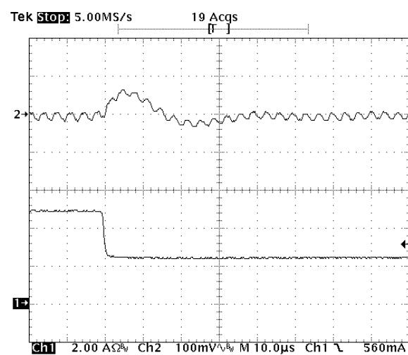
**Fig-1.8V-7:** Output voltage response for  $V_{out}=1.8V$  to positive load current step-change from 5A to 2.5A with slew rate of  $-5A/\mu s$  at  $V_{in}=5.0V$ .  $C_o=47\mu Fx2$  ceramic.
