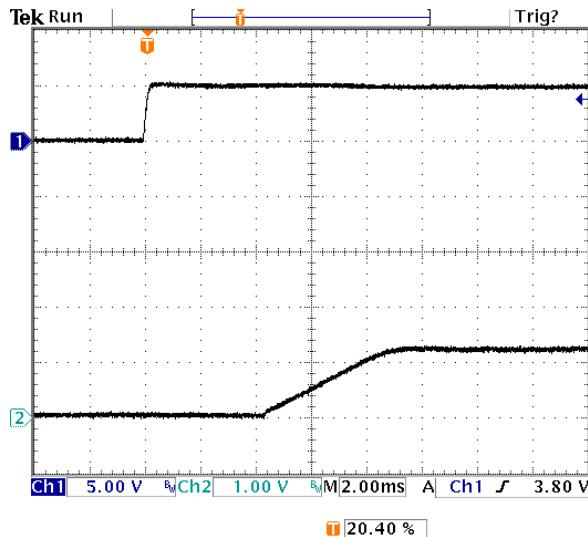
**Fig-1.2V-4:** Turn-on transient for  $V_{out}=1.2V$  with application of  $V_{in}$  at full rated load current (resistive) and  $47\mu Fx2$  external capacitance at  $V_{in}=5.0V$ .
