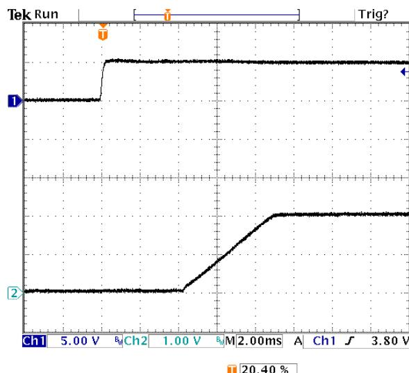
**Fig-2.0V-4:** Turn-on transient for  $V_{out}=2.0V$  with application of  $V_{in}$  at full rated load current (resistive) and  $47\mu Fx2$  external capacitance at  $V_{in}=5.0V$ .
