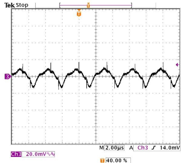
**Fig-1.2V-5:** Output voltage ripple (20mV/div.) for  $V_{out}=1.2V$  at full rated load current into a resistive load with external capacitance  $47\mu Fx2$  ceramic +  $1\mu F$  ceramic at  $V_{in}=5.0V$ .
