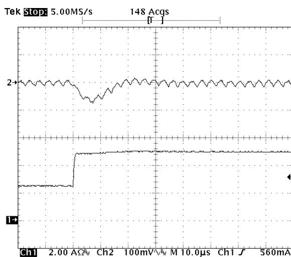
**Fig-1.5V-6:** Output voltage response for  $V_{out}=1.5V$  to positive load current step-change from 2.5A to 5A with slew rate of  $5A/\mu s$  at  $V_{in}=5.0V$ .  $C_o=47\mu Fx2$  ceramic.
