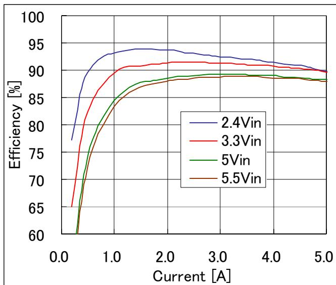
**Fig-1.5V-2:** Efficiency vs. load current and input voltage for  $V_{out}=1.5V$ .
