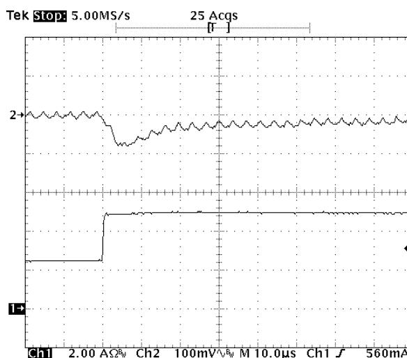
**Fig-3.3V-6:** Output voltage response for  $V_{out}=3.3V$  to positive load current step-change from 2.5A to 5A with slew rate of  $5A/\mu s$  at  $Vin=5.0V$ .  $Co=47\mu Fx2$  ceramic.
