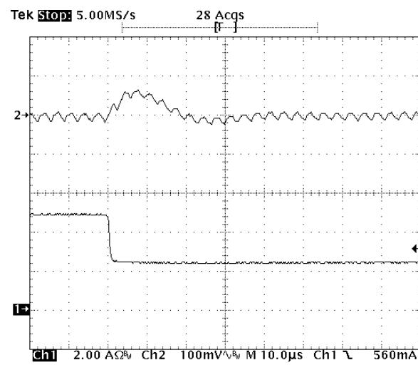
**Fig-1.5V-7:** Output voltage response for  $V_{out}=1.5V$  to positive load current step-change from 5A to 2.5A with slew rate of  $-5A/\mu s$  at  $V_{in}=5.0V$ .  $C_o=47\mu Fx2$  ceramic.
