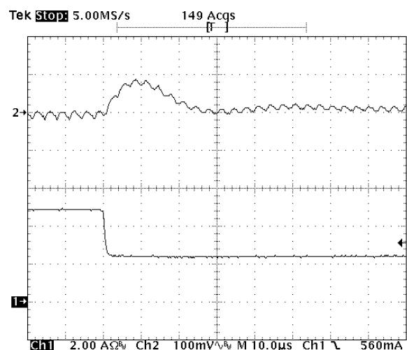
**Fig-2.5V-7:** Output voltage response for  $V_{out}=2.5V$  to positive load current step-change from 5A to 2.5A with slew rate of  $-5A/\mu s$  at  $V_{in}=5.0V$ .  $C_o=47\mu Fx2$  ceramic.
