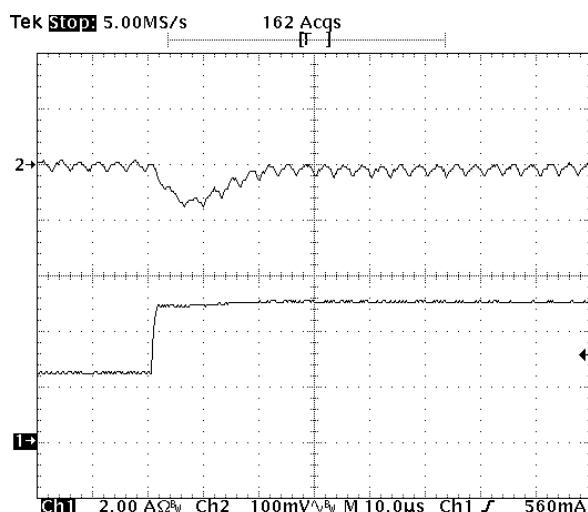
**Fig-1.2V-6:** Output voltage response for  $V_{out}=1.2V$  to positive load current step-change from  $2.5A$  to  $5A$  with slew rate of  $5A/\mu s$  at  $V_{in}=5.0V$ .  $C_o=47\mu Fx2$  ceramic.
