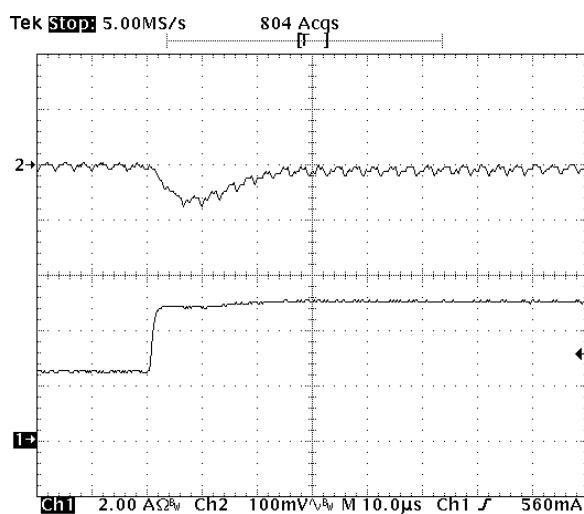
**Fig-0.7525V-6:** Output voltage response for  $V_{out}=0.7525V$  to positive load current step-change from  $2.5A$  to  $5A$  with slew rate of  $5A/\mu s$  at  $V_{in}=5.0V$ .  $C_o=47\mu Fx2$  ceramic.
