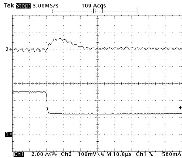
**Fig-0.7525V-7:** Output voltage response for  $V_{out}=0.7525V$  to positive load current step-change from  $5A$  to  $2.5A$  with slew rate of  $-5A/\mu s$  at  $V_{in}=5.0V$ .  $C_o=47\mu Fx2$  ceramic.
