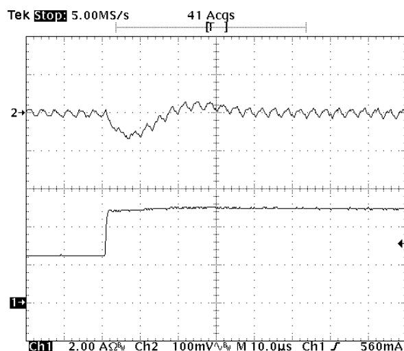
**Fig-2.0V-6:** Output voltage response for  $V_{out}=2.0V$  to positive load current step-change from 2.5A to 5A with slew rate of  $5A/\mu s$  at  $V_{in}=5.0V$ .  $C_o=47\mu Fx2$  ceramic.
