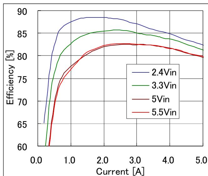
**Fig-0.7525V-2:** Efficiency vs. load current and input voltage for  $V_{out}=0.7525V$ .
