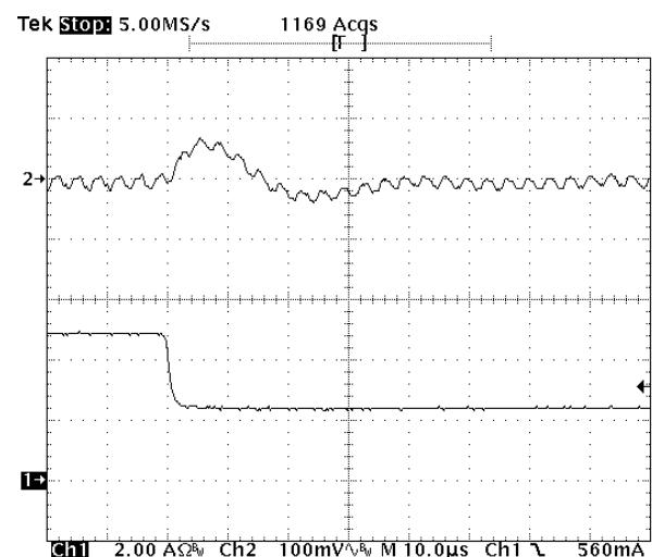
**Fig-2.0V-7:** Output voltage response for  $V_{out}=2.0V$  to positive load current step-change from 5A to 2.5A with slew rate of  $-5A/\mu s$  at  $V_{in}=5.0V$ .  $C_o=47\mu Fx2$  ceramic.
