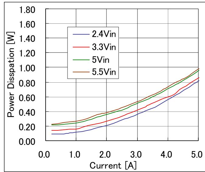
**Fig-1.2V-3:** Power dissipation vs. load current and input voltage for  $V_{out}=1.2V$ . Airflow rate=200 LFM (1.0m/s) and  $T_a=25^{\circ}C$ .
