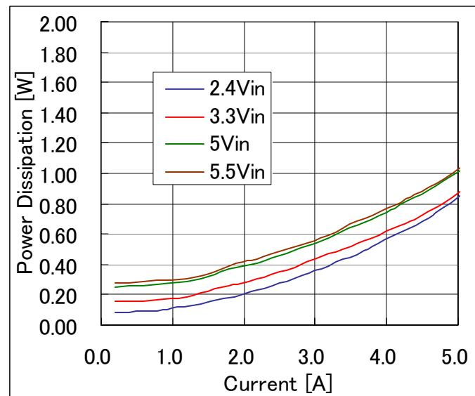
**Fig-1.5V-3:** Power dissipation vs. load current and input voltage for  $V_{out}=1.5V$ .
