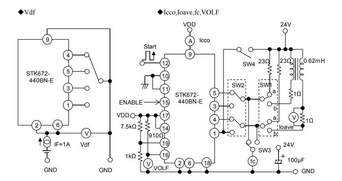
Ioave measurement: Set switch SW2 in the setting SW1 to 'b'.
