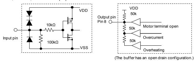
The input pins of this driver all use Schmitt input. Typical specifications at Tc=25°C are given below. Hysteresis voltage is 0.3V (VIHa-VILa).
