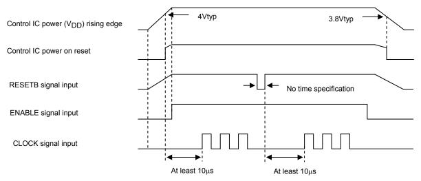
ENABLE, CLOCK, and RESETB Signals Input Timing
