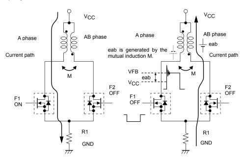
The oscillating voltage in excess of VFB is caused by LCRM (inductance, capacitor, resistor, mutual inductance) oscillation that includes micro capacitors C, not present in the circuit. Since M is affected by the motor characteristics, there is some difference in oscillating voltage according to the motor specifications. In addition, constant voltage drive without constant current drive enables motor rotation at  $V_{CC} \ge 0V$ .
