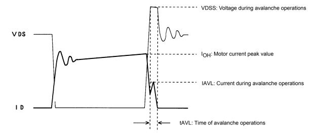
Figure 1 Output Current, I<sub>D</sub>, and Voltage, V<sub>DS</sub>, Waveforms 1 of the STK672-4\*\* Series when Driving a 2-Phase Stepper Motor with Constant Current Chopping
