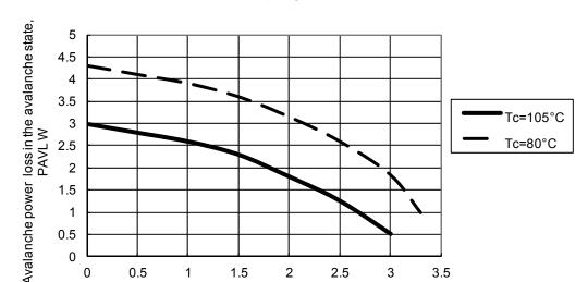
Figure 3 Allowable Loss Range, PAVL-I<sub>OH</sub> During STK672-440BN-E Avalanche Operations PAVL-IOH
