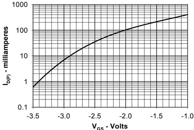
Fig. 4. Plateau current versus applied input voltage
