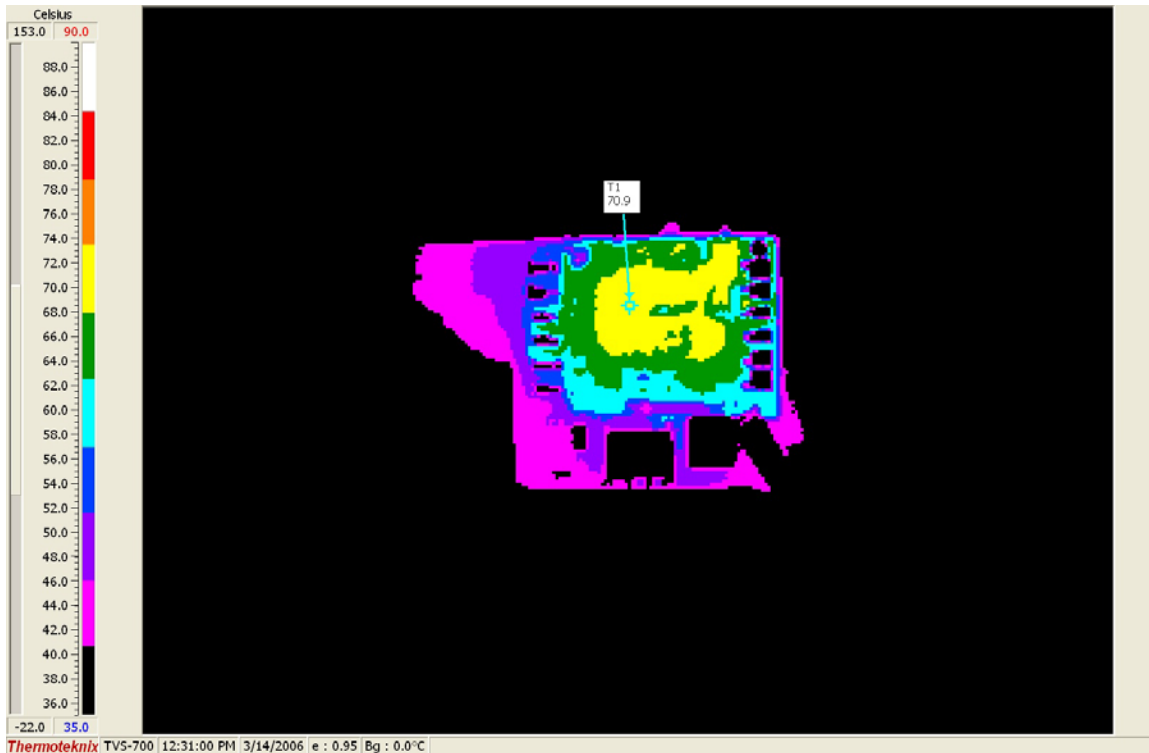
Figure 7. Temp Data (48Vin, 5A, 100LFM airflow – front)
