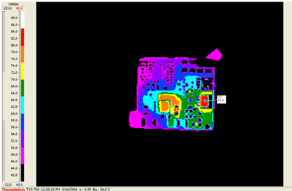
Figure 8. Temp Data (48Vin, 8A, 100LFM airflow – back)
