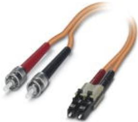
Assembled FO cable, zip cord cable, multi-mode fiberglass 50/125  $\mu\text{m}$ , OM2, plug: LC/B-FOC (ST), degree of protection: IP20, for installation in cable ducts or control cabinets, length: 1 m
