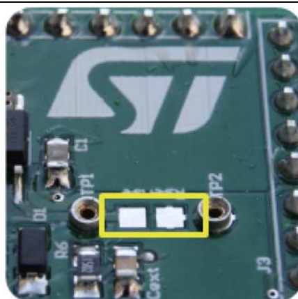
Figure 5. Pads for soldering SMD resistor
