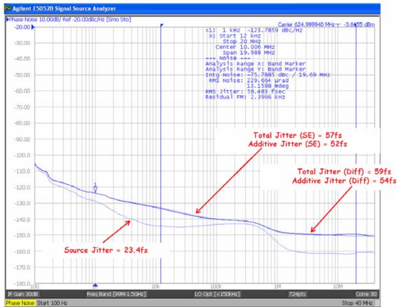
Figure 2.15. Total Jitter Differential Input (312.5 MHz)
