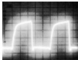
Signal Waveform (20ns/div / 1V/div)
