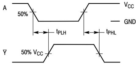
Figure 3. Switching Waveforms
