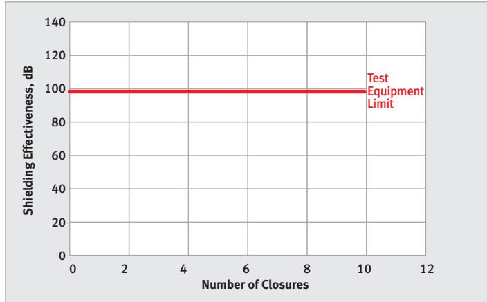
Tested in accordance with ARP 1705 (mod) at 1 GHz.
