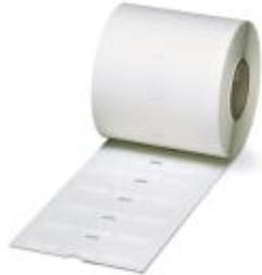
Cable marker label, Roll, white, Unlabeled, Can be labeled with: Thermomark R, Thermomark X, Thermomark S, Mounting type: Adhesive, Cable diameter:  $\leq 7.5$  mm, Lettering field: 25 x 13 mm
