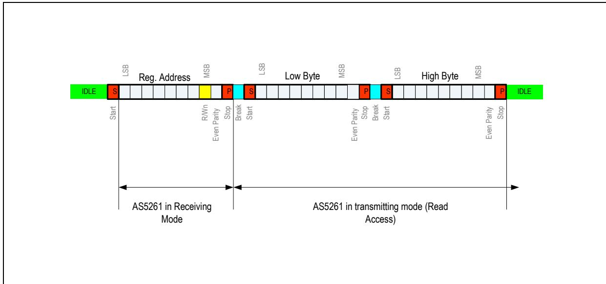
The R/Wn bit in the first byte selects the mode. Between the data packets is always a break state. The break state has the same length as the other data bits.
