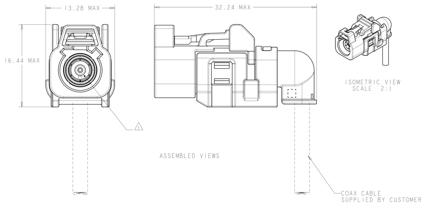
1. PLUG ACCEPTS JACKS MEETING DIN 72594-1, ROAD VEHICLES - RADIO FREQUENCY INTERFACE - DIMENSIONS AND ELECTRICAL REQUIREMENTS.
