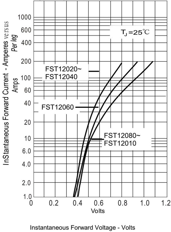
Figure .2-Forward Derating Curve
