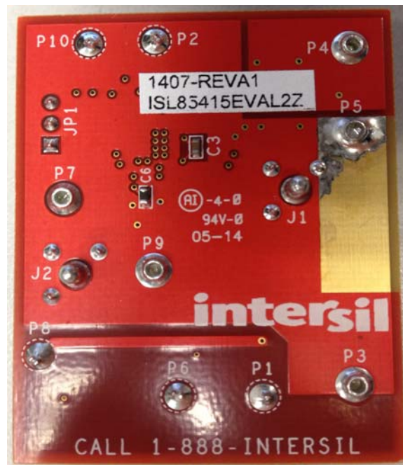
FIGURE 2. BACK OF EVALUATION BOARD ISL85415EVAL2Z
