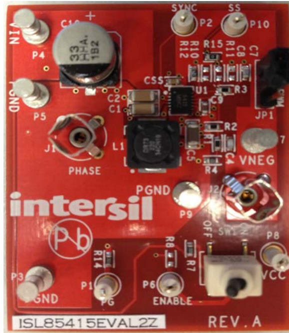
FIGURE 1. FRONT OF EVALUATION BOARD ISL85415EVAL2Z
