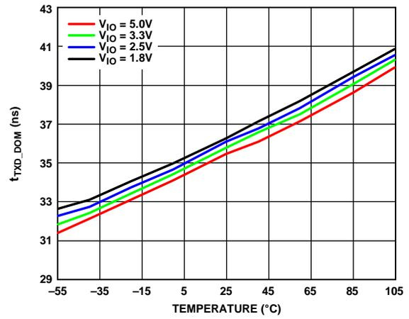
Figure 14.  $t_{TXD\_DOM}$  vs. Temperature
