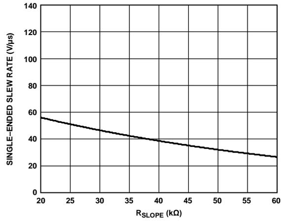
Figure 12. Single-Ended Slew Rate vs.  $R_{SLOPE}$
