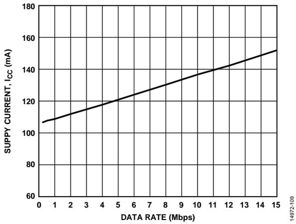
Figure 10. Supply Current,  $I_{CC}$  vs. Data Rate
