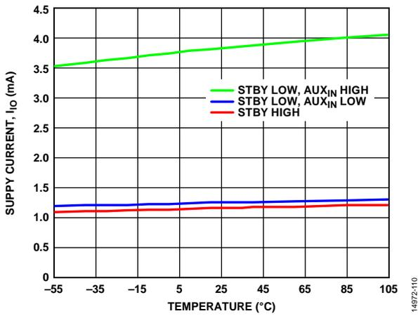
Figure 11. Supply Current,  $I_{IO}$  vs. Temperature (Inputs Idle)
