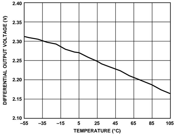
Figure 20. Differential Output Voltage ( $V_{OD}$ ) vs. Temperature
