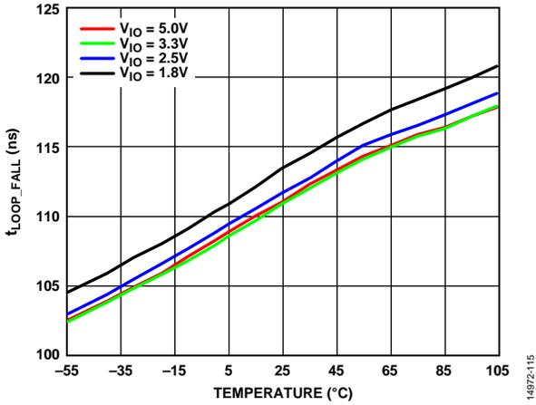
Figure 16.  $t_{LOOP\_FALL}$  vs. Temperature ( $R_{SLOPE} = 0 \Omega$ )
