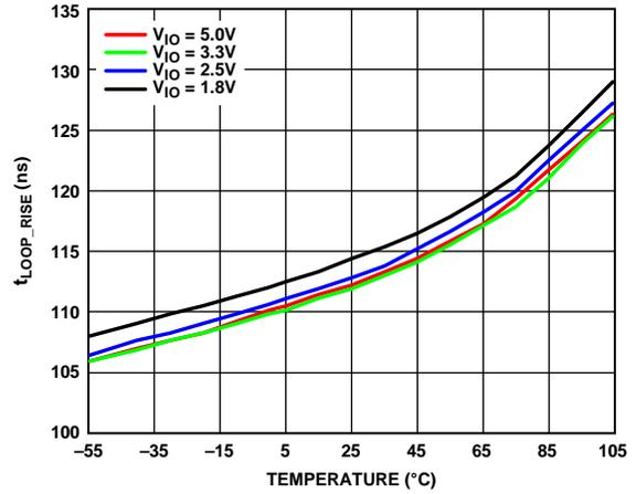
Figure 18.  $t_{LOOP\_RISE}$  vs. Temperature ( $R_{SLOPE} = 0 \Omega$ )
