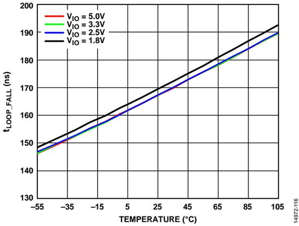
Figure 17.  $t_{LOOP\_FALL}$  vs. Temperature ( $R_{SLOPE} = 47 \text{ k}\Omega$ )
