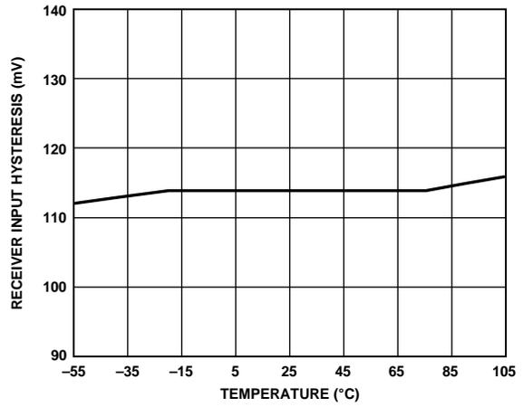
Figure 13. Receiver Input Hysteresis vs. Temperature
