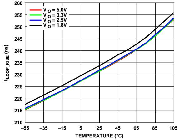
Figure 19.  $t_{LOOP\_RISE}$  vs. Temperature ( $R_{SLOPE} = 47 \text{ k}\Omega$ )
