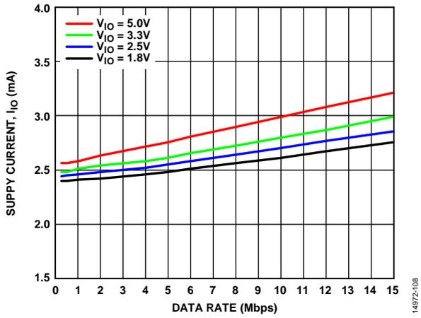
Figure 9. Supply Current,  $I_{IO}$  vs. Data Rate
