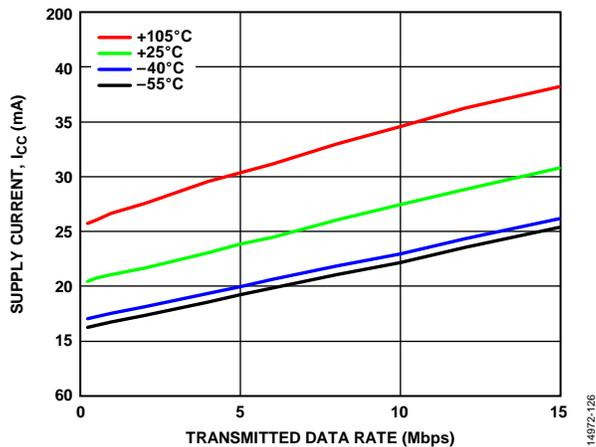
Figure 27. Supply Current,  $I_{CC}$  vs. Transmitted Data Rate
