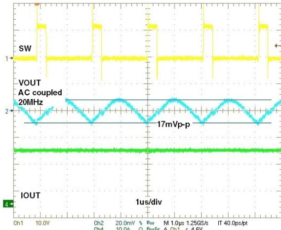
Figure 13: Steady state, CCM,  $I_{OUT} = 20A$
