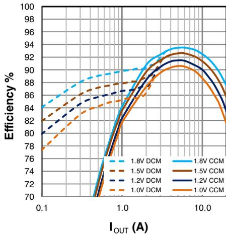
Figure 19: Efficiency,  $V_{IN}=5\text{V}$
