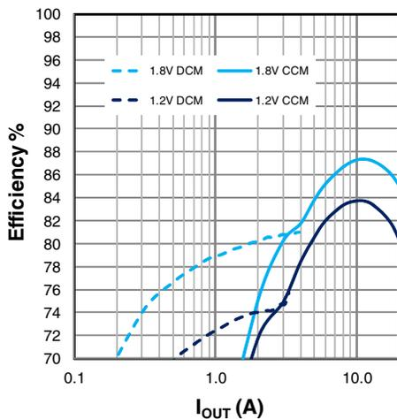
Figure 23: Efficiency,  $V_{IN}=19.6\text{V}$
