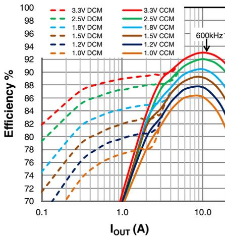
Figure 21: Efficiency,  $V_{IN}=12\text{V}$
