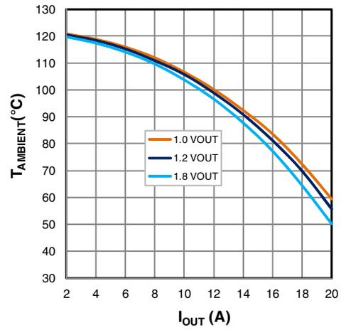
Figure 20: Maximum  $T_{AMBIENT}$  vs  $I_{OUT}$ ,  $V_{IN}=5\text{V}$
