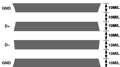
Figure 34. Arrangement of Signal Tracks
