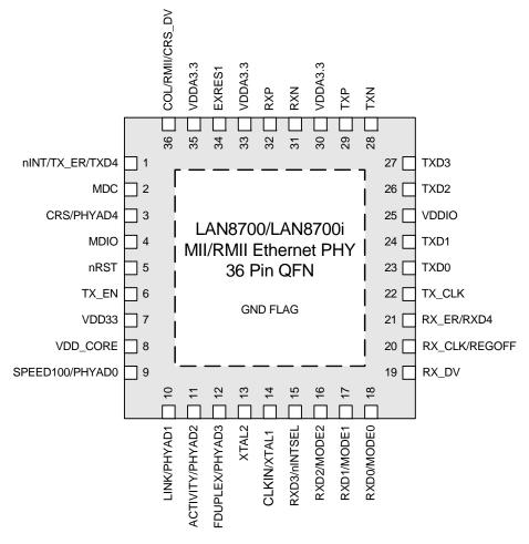
Figure 2.1 Package Pinout (Top View)
