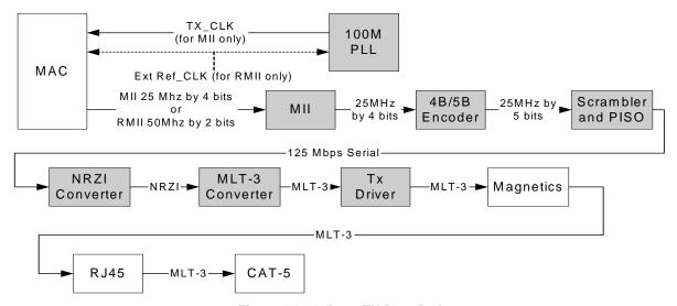
Figure 4.1 100Base-TX Data Path
