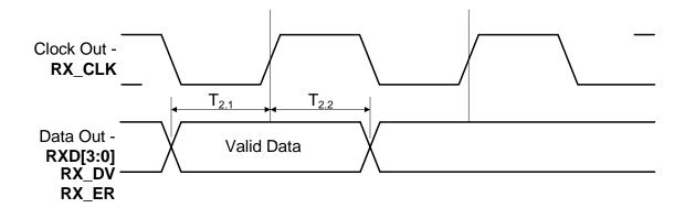
Figure 6.2 100M MII Receive Timing Diagram
