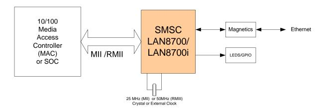
Figure 1.1 LAN8700/LAN8700i System Block Diagram
