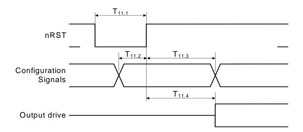
Figure 6.10 Reset Timing Diagram
