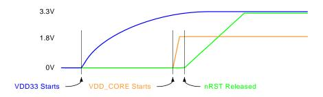
Figure 5.1 Reset Timing Diagram
