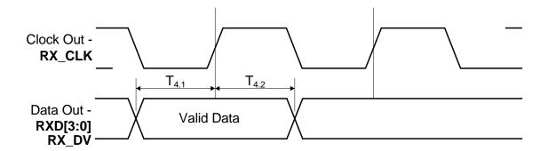
Figure 6.4 10M MII Receive Timing Diagram
