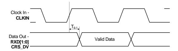
Figure 6.8 10M RMII Receive Timing Diagram
