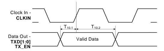
Figure 6.9 10M RMII Transmit Timing Diagram
