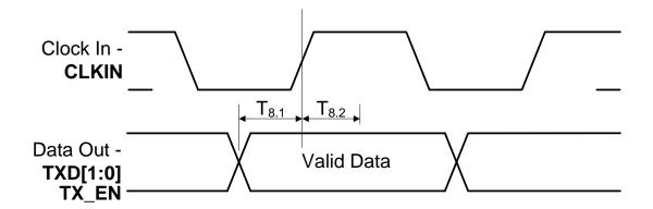
Figure 6.7 100M RMII Transmit Timing Diagram
