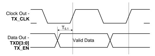
Figure 6.5 10M MII Transmit Timing Diagrams
