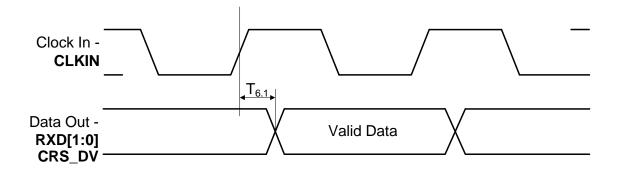
Figure 6.6 100M RMII Receive Timing Diagram
