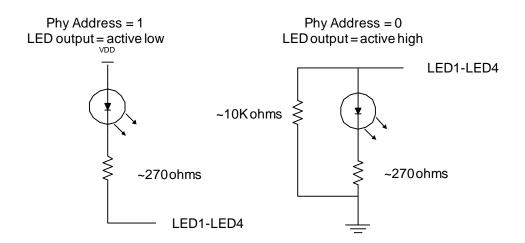
Figure 4.5 PHY Address Strapping on LED's
