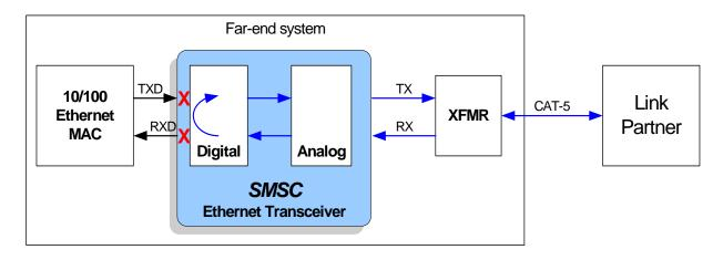
Figure 5.3 Far Loopback Block Diagram
