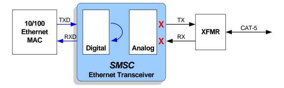
Figure 5.2 Near-end Loopback Block Diagram
