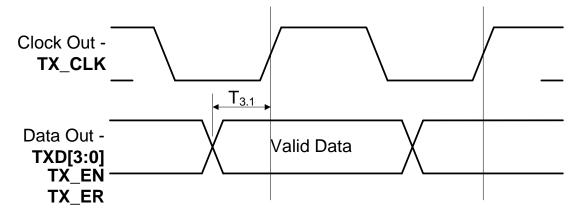
Figure 6.3 100M MII Transmit Timing Diagram
