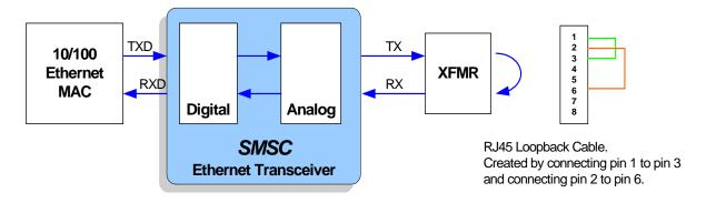
Figure 5.4 Connector Loopback Block Diagram
