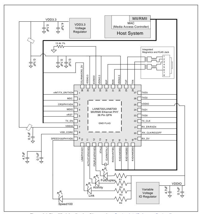
Figure 8.1 Simplified Application Diagram (see Section 8.4, "Reference Designs")
