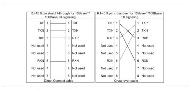
Figure 4.4 Direct Cable Connection vs. Cross-over Cable Connection.
