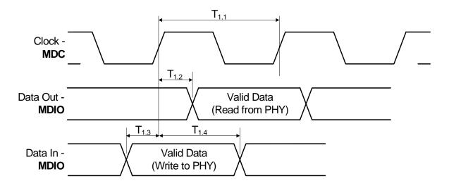
Figure 6.1 SMI Timing Diagram
