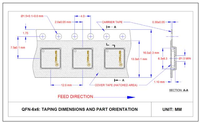
Figure 9.2 QFN, 6x6 Tape & Reel
