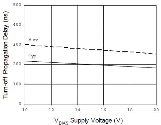
Figure 5B. Turn-off Propagation Delay
