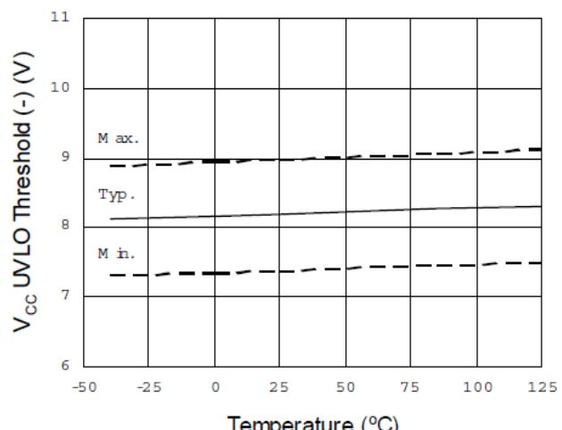
Figure 18.  $V_{CC}$  Undervoltage Threshold (-)
