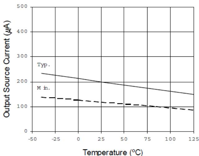
Figure 21A. Output Source Current
