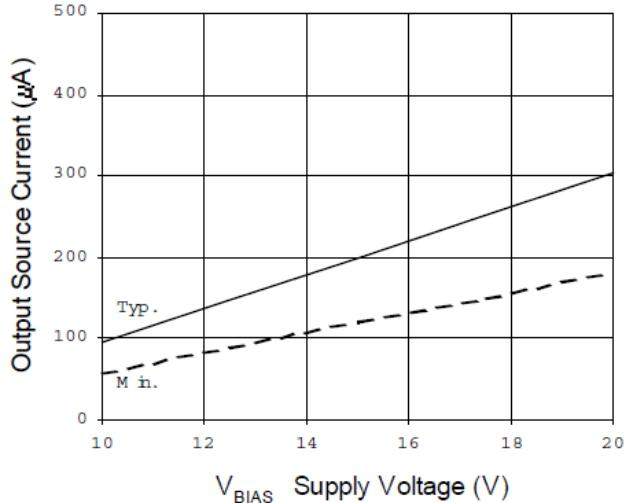
Figure 21B. Output Source Current
