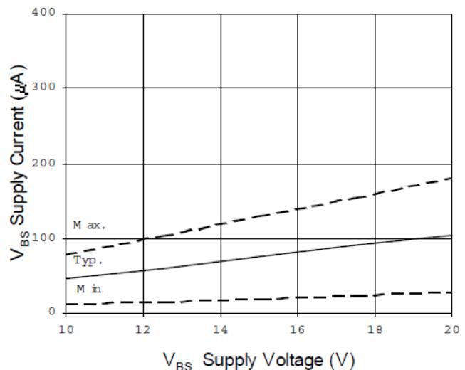
Figure 13B. V<sub>BS</sub> Supply Current vs. Supply Voltage
