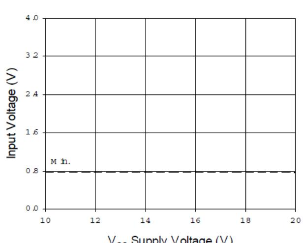
Figure 9B. Logic "0" Input Voltage
