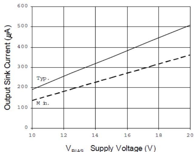
Figure 22B. Output Sink Current vs. Supply Voltage
