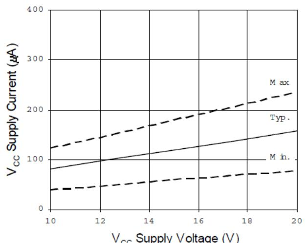
Figure 14B. Quiescent V<sub>CC</sub> Supply Current vs. V<sub>CC</sub> Supply Voltage
