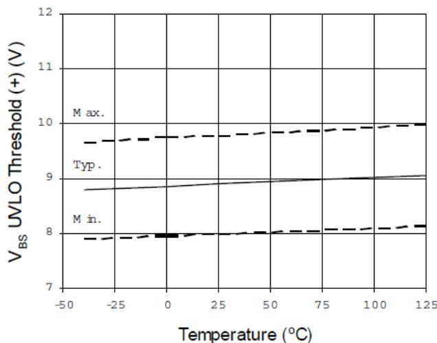
Figure 19.  $V_{BS}$  Undervoltage Threshold (+)
