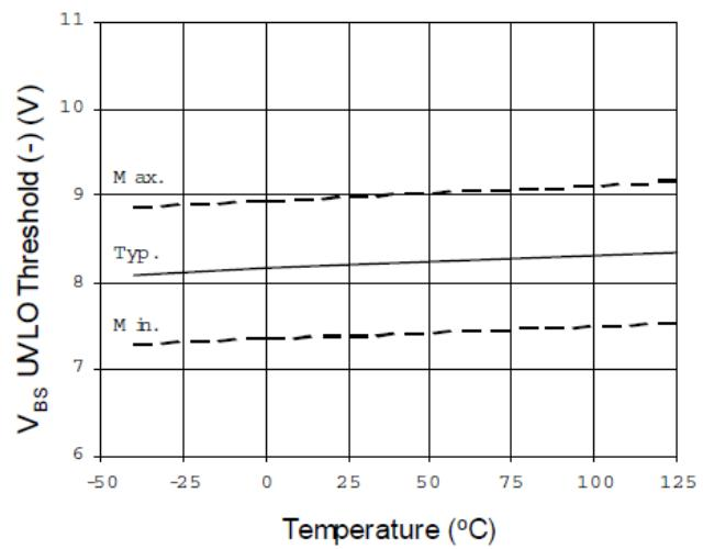
Figure 20.  $V_{BS}$  Undervoltage Threshold (-)
