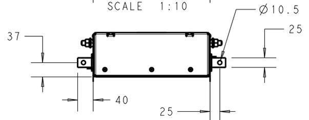
\* DO NOT LOOSEN INNER GROUND NUTS. TORQUE OUTER GROUND NUTS TO: 25-30 NM [220-260 IN-LB]
