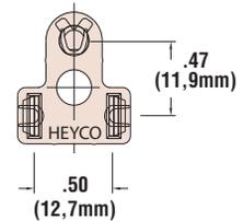
.050 REC. OVERMOLD THICKNESS ON FACE
