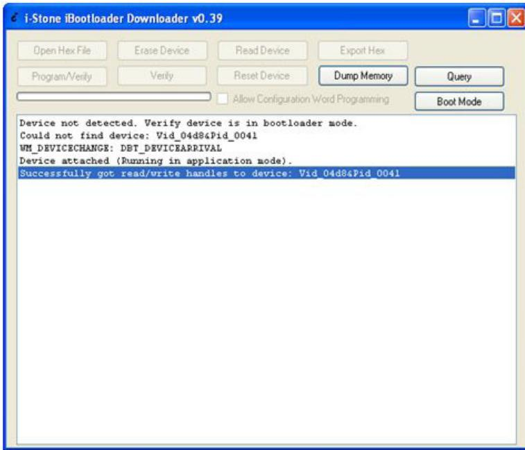
Figure 17. Alignment box detected running in application mode
