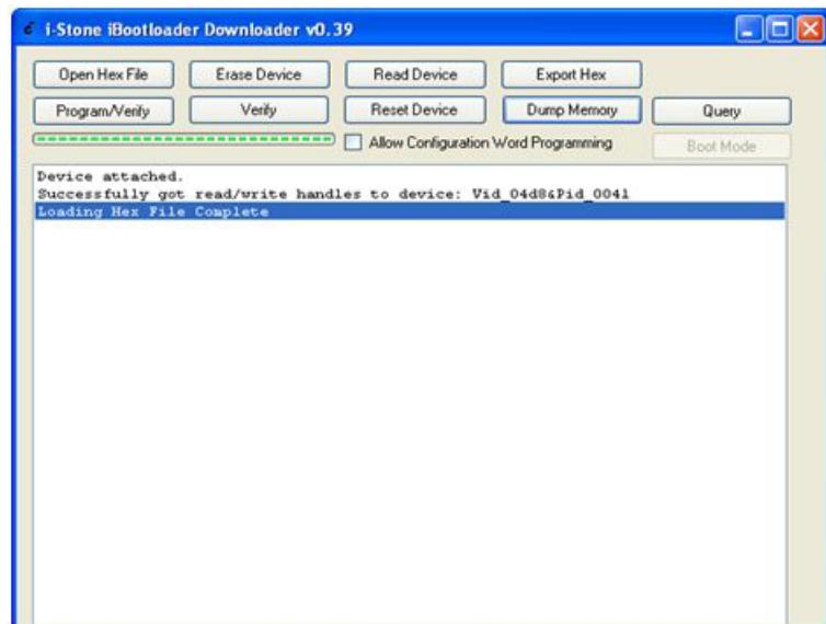
Figure 20. Program verify process and upon completion of Hex file.
