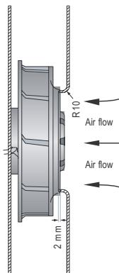
The air flow and noise level of fans without external housing depends on the installation conditions. The stated air flow and noise has been measured under the following conditions:
