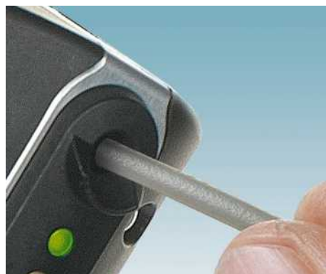
... stripping and crimping is carried out automatically, ...
