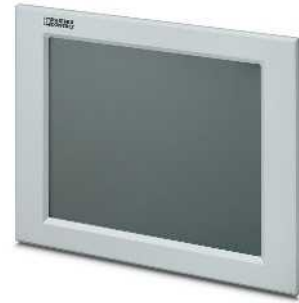
Panel PC with Atom™ processor
