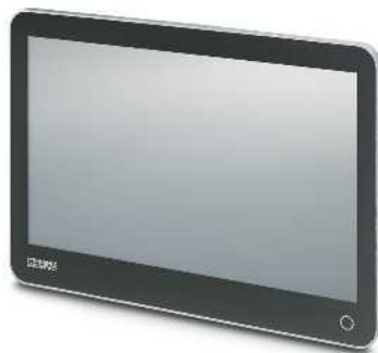
Fully enclosed IP65 IPC with 54.6 cm (21.5") display
