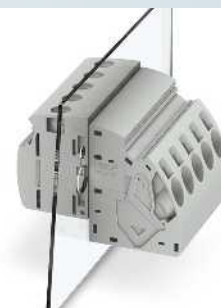
16 mm 2 panel feed-through terminal block, external part with push-in connection, internal part with screw connection
