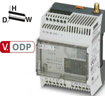
Communication via ODP protocol, 2 additional analog inputs
